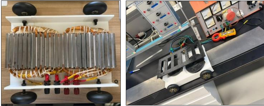
Figure 2. Fabricated Prototype Shuttle: Hand-Wound 4-Pole Primary In The PETG Carriage On Polyurethane Wheels Over The Aluminium Reaction Plate.
